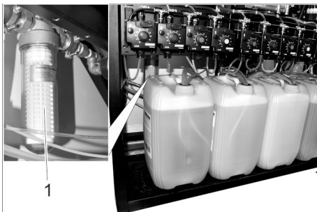
1 Filter for frost-protection pump
